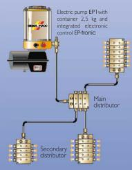
The electronic control of the central lubrication is adapted to the operating conditions of the vehicle and activates the pump in the fixed interval.
